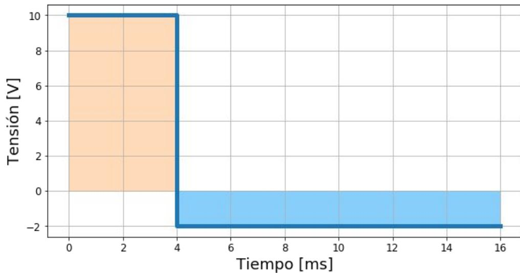
$$V_{DC} = 1 \text{ V}$$
