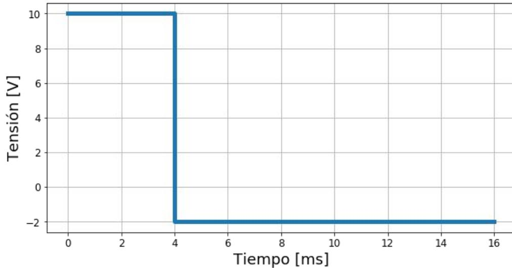
$$V_{ef} = \sqrt{\frac{1}{T} \int_0^T v^2(t) dt}$$
