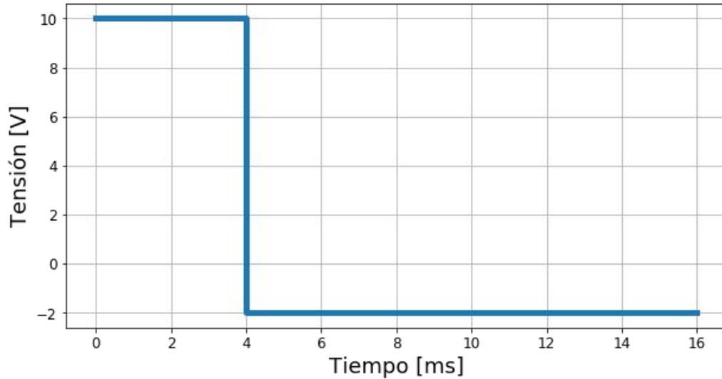
$$V_{ef} = \sqrt{\frac{1}{T} \int_0^T v^2(t) dt}$$
