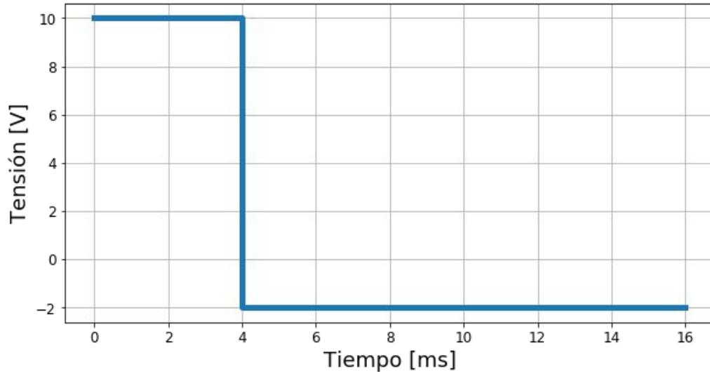
$$V_{DC} = \frac{1}{T} \int_0^T v(t) dt$$
