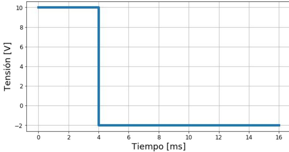
$$V_{ef} = 5.29 \text{ V}$$
