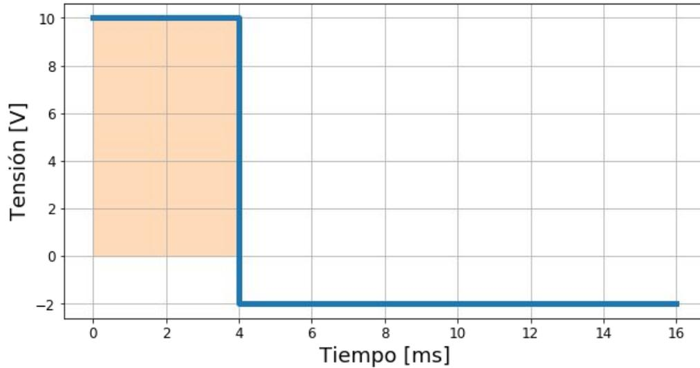
$$V_{DC} = \frac{1}{16 \text{ ms}} (10 \text{ V} \cdot 4 \text{ ms})$$
